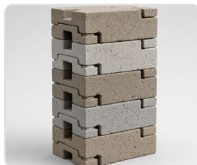
1. Sintered regolith blocks
