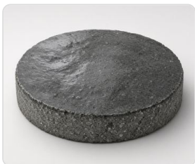
2. Microwave-glazed floor and landing pad
